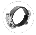
In this version, the ends of the brackets are folded back and spotwelded onto the band. Thanks to its structure the NORMACLAMP<sup>®</sup> HMK two-parts is suitable for use with even high mechanical loads and for retaining extremely heavy pipes and connectors.
