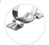
These are prefabricated brackets which you can use to transform NORMACLAMP® standard clamps (types GBS, HD, SP and TORRO) into retaining clamps with brackets in no time at all. Just open the standard clamp, guide the band through the bracket slot, and that's all there is to it.
